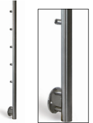
XL4421205M AISI 316 polished tube Ø 42,4 x 2,0 mm Height 1200 mm
